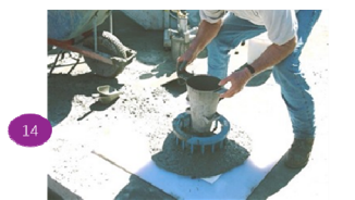
A trial mix of Grade C45/10 concrete with minimum slump of 100mm
